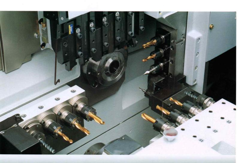
**CNC Swiss Type Automatic Lathe**
